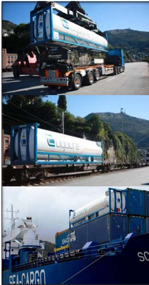
Figure 2: Liquline has experience with transporting LNG via ISO containers on trucks (top), trains (middle) and ships (bottom). Photo courtesy of Liquline.
